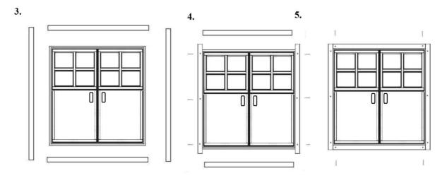
Then insert door frame in to its space from the outside of the structure and attach the rest of the support trims form inside the structure.
