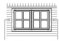
Just insert the window frame in to the space (no screwing)
