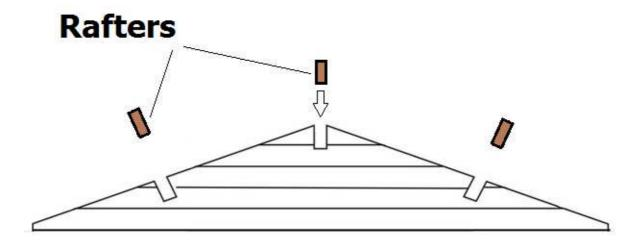
**4.7. Roof-boards:** The next step is to attach the roof-boards vertically and screw them into the rafters. Make sure the ends of the roof-boards are perfectly parallel to each other. Then fix the roof plank boarder under the roof-boards as show below. The roof-plank must be screwed to the roof plank boarder.
